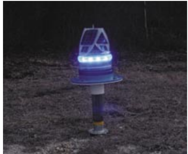
AV70-B model being tested by FAA for "Remote Airfield Lighting". New Jersey testing facility (USA)
