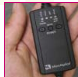
Belt-Worn Battery Dimensions: 3" x 2" x 0.5"
