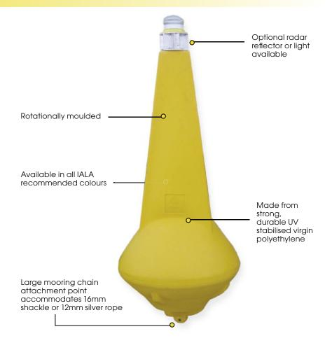
The SLB700 is a short-range buoy ready for immediate installation. Typical applications include day and night channel, speed zone, restricted area marking and aquaculture.
